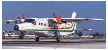
The Hindustan-228 aircraft is a multi-purpose, light-weight, twin turboprop aircraft. It has been indigenised by HAL to operate on short haul air routes under the regional connectivity scheme UDAN
