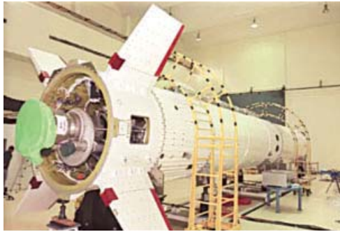
Test vehicle for characterisation of Crew Escape System ready at SDSC
